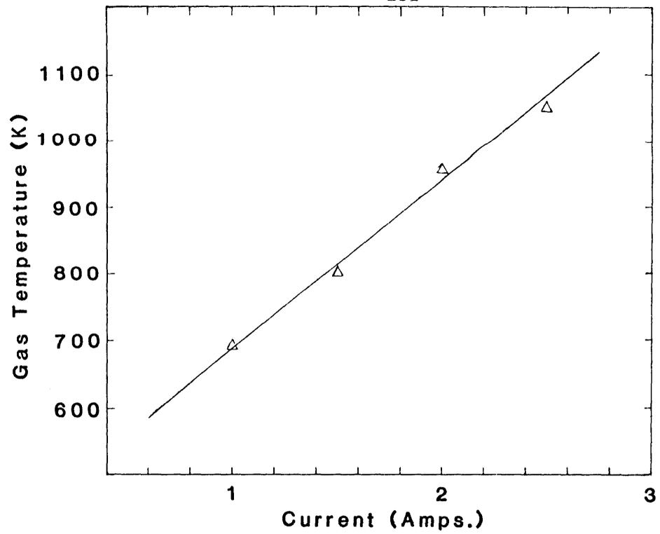
Figure A2.3 Plot of the measured value of the gas temperature versus discharge current in a "pure" helium hollow cathode discharge at a constant pressure of 20 Torr
