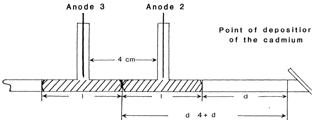
Figure A3.1 Schematic diagram defining the parameters used in the analysis of the cadmium ground state density absorption experiment
