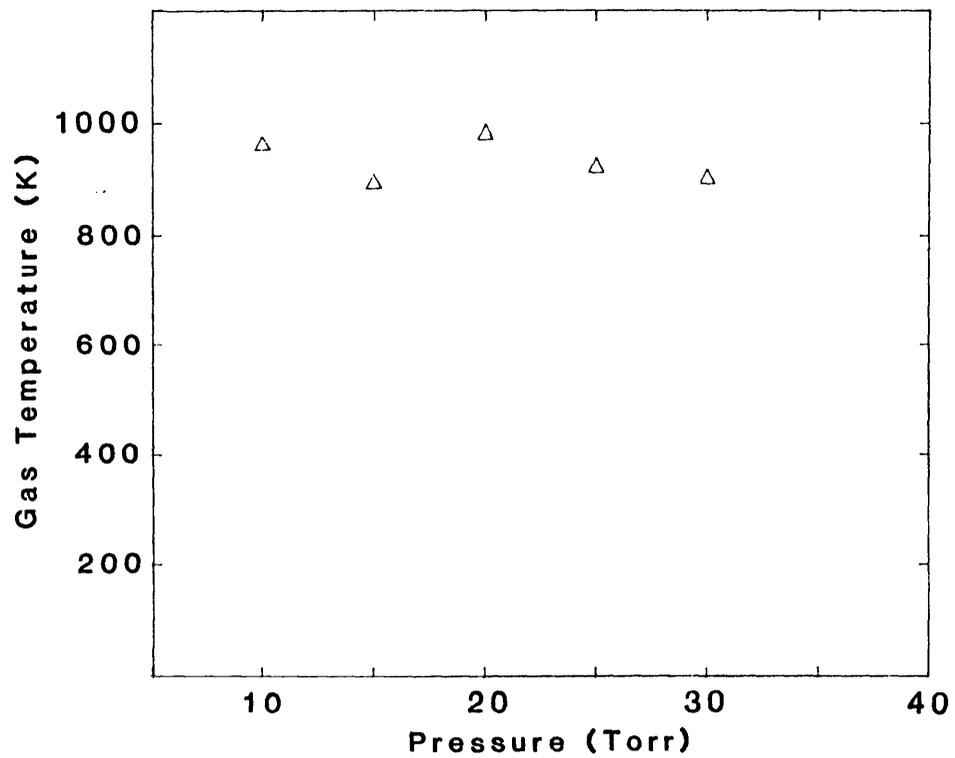
Figure A2.4 Plot of the measured values of the gas temperature versus helium pressure at a constant current of 120 mA/anode
