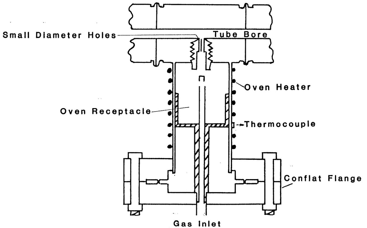
Figure A1.4 Design of the oven section of the laser tube
