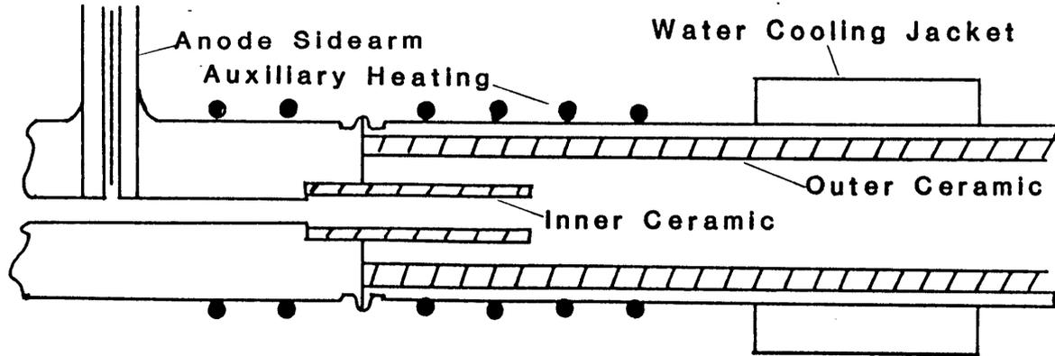
Figure A1.3 Design of the endpiece of the laser tube
