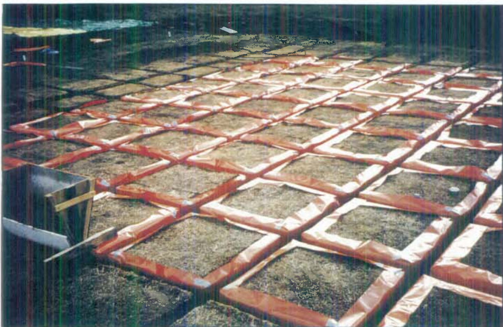
Plate 3.2: The soil 'islands' were individually wrapped in construction grade plastic before the trenches were back-filled with soil. The plastic sheeting was used to prevent water and root movement between plots.
