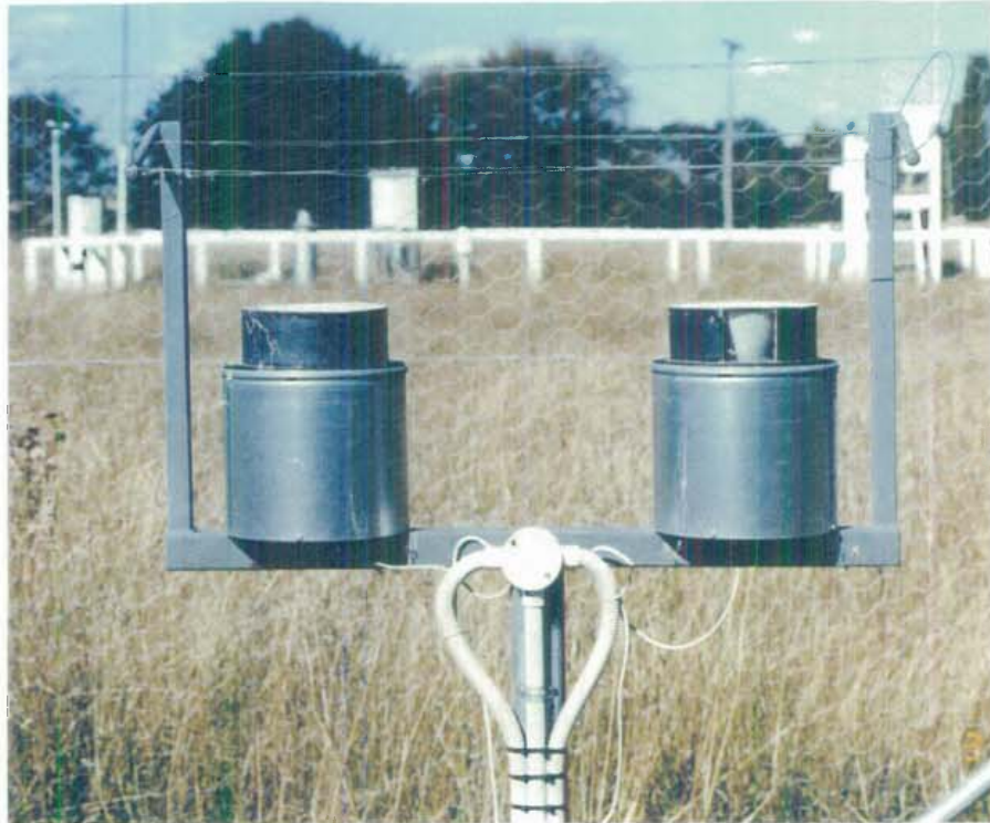
Plate 3.3: Two tipping rain gauges measured the rainfall. When 0.25 mm was received in either rain gauge the tipping mechanism caused an electronic pulse to be sent to the controller. The second rain gauge was installed as a backup in case of malfunction or blockage.
