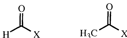
Figure 10.3 Structures containing formyl and acetyl groups of interest in the present research, where X = H, OH, F, Cl, Br, NH 2 etc.
