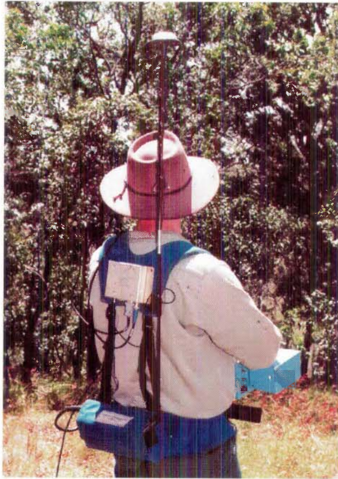
Plate 7-1. The TM-4 based SAM Receiver showing the mounting position of the Trimble SVeeSix GPS Receiver.
