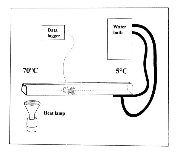
Figure 2.1. Temperature gradient apparatus used for measuring temperature selection in *Urodacus manicatus* showing one track of eight.
