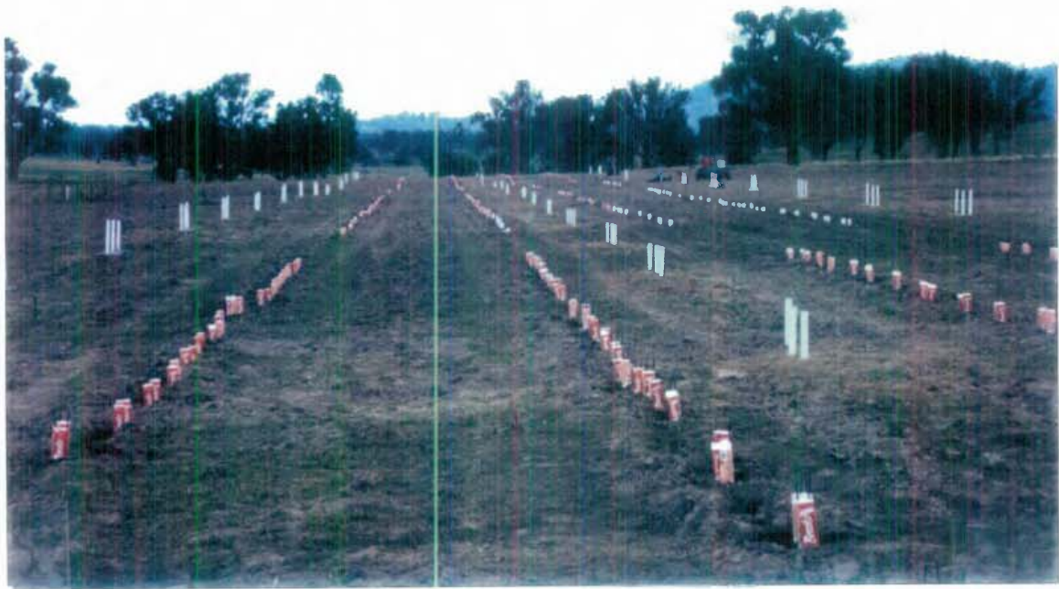
Plate 2a. Showing the established experimental site at Tullimba. Planted trees were protected with milk cartons around them. Observation wells (each instrument station including 3 wells) were established above, within and below the experimental zone.
