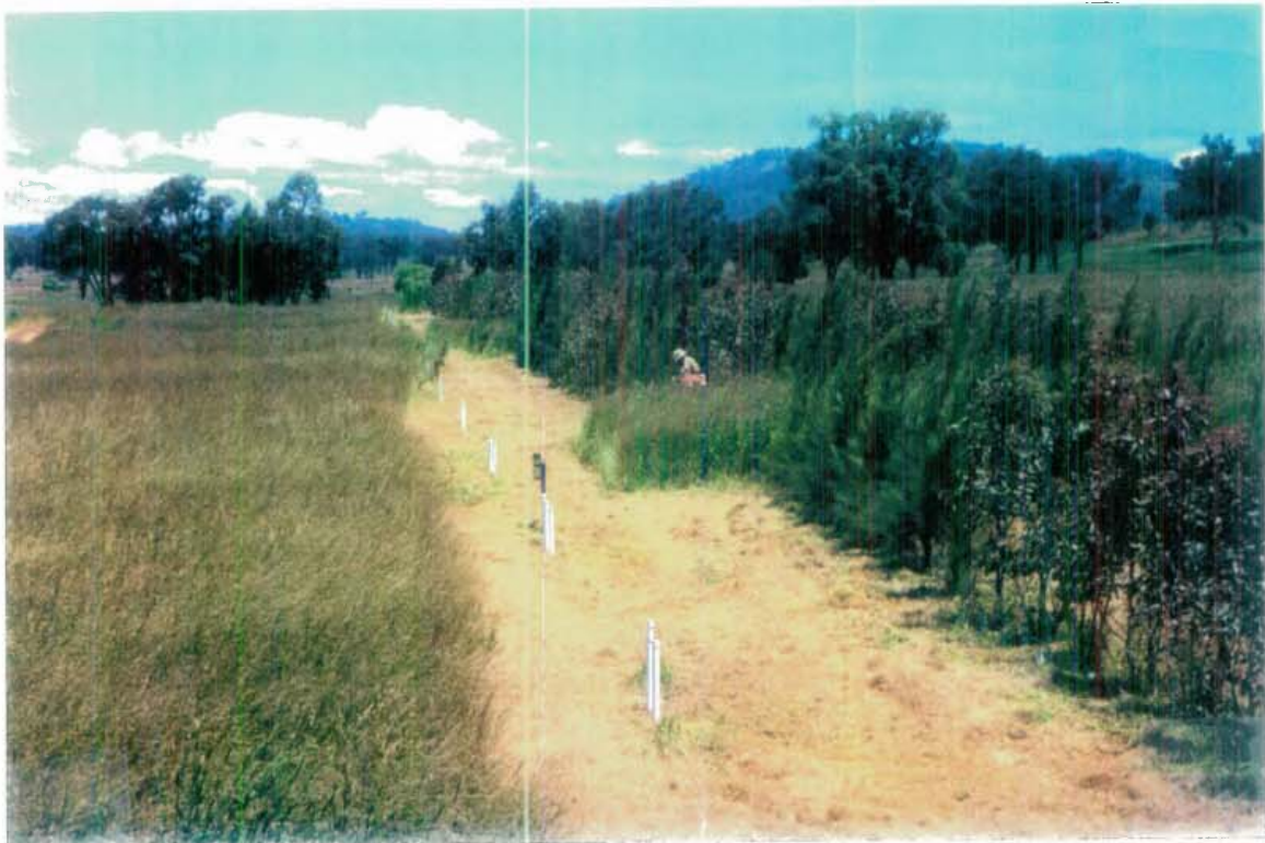
Plate 2a. Showing the established experimental site at Tullimba. Planted trees were protected with milk cartons around them. Observation wells (each instrument station including 3 wells) were established above, within and below the experimental zone.
