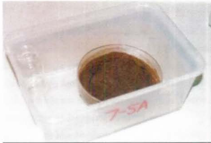
Figure 4.3: Biological incubation chamber, with topsoil and KOH in the clear vial.
