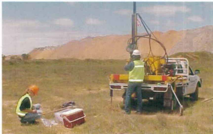
Figure 5.9: Truck-mounted soil corer at Cheshunt mine collecting 6 m stockpile samples.
