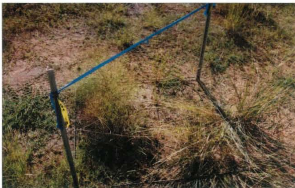
Figure 5.11: Vegetation monitoring using a 1 m by 1 m quadrat.
