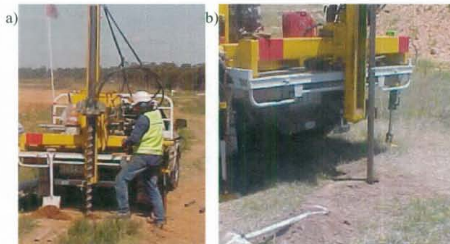
Figure 5.10: Truck-mounted soil corer (a) showing auger head and (b) push tube interchange capabilities.
