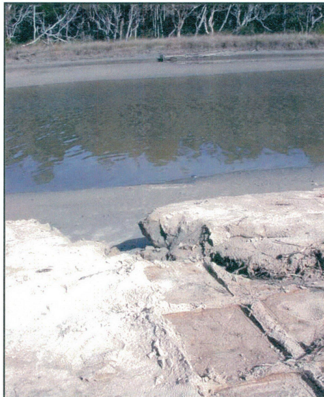
Fig. 6.3.4 The original positions of some of the experimental trays can be seen in the bottom-right corner. At the time of deployment, this area was covered by 0.6 m of water. In this case, both sediment scouring and a large reduction in waterway area has occurred following entrance closure.
