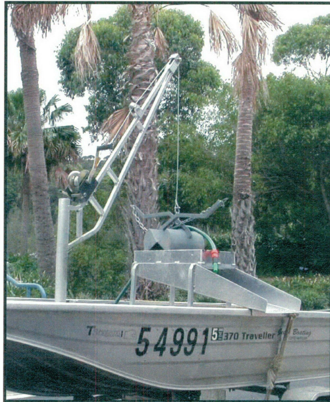
Fig. 2.4.1a View of sampling equipment including grab, gantry/winch, sieve and wash tray.
