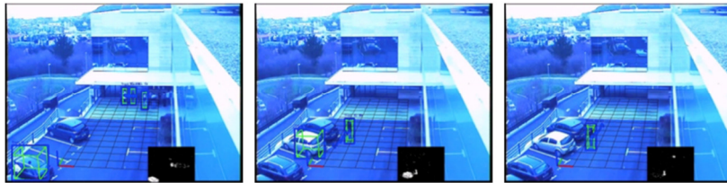
Figure 7: Detection of Cars and People can be used to create interaction rules, such as “Person Out of Car”.
