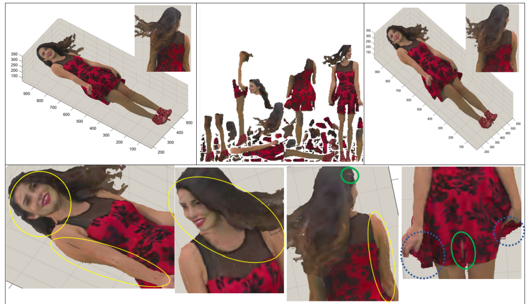
Figure 3. Different artefacts appear because of data loss while encoding by V-PCC, where a Redundant-black video frame is used.
