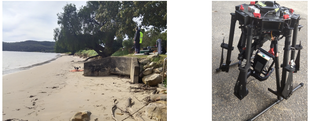
Figure 5. Trial site preparations. (left) The beach where we performed our in flight tests. (right) The completed DAQ and camera mounted on a gimbal ready to be deployed. The GNSS antenna was carefully routed to the top.
