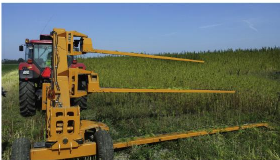
Fig. 3. Tebeco Clipper 4.3 MMH—the stems sections are left onto the ground occupying the full field area.
