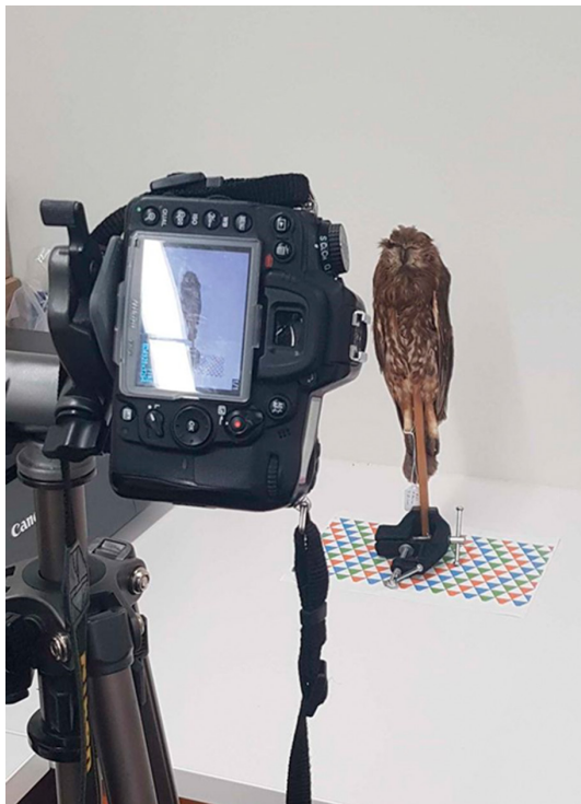
FIGURE 3 A taxidermized Southern Boobook ( Ninox boobook ) being photographed to create a digital model that can be 3D-printed and used to create a printed 'texture'. The model was rotated by gently turning the clamp and paper sheet between photographs. We used a paper sheet covered in colored triangles, as we found this improved the alignment of the photographs.
