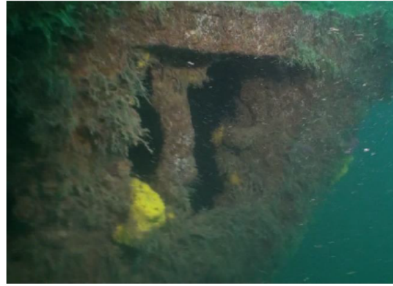
Figure 46. Gaps in hull plating at the stern of the wreck mimic hatches. 2012
