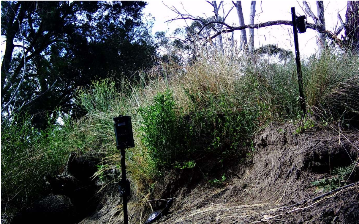
Figure 3.2 - Example of inward-facing camera trap (below) with ultrasonic repellent device (top of stake) at an impact site (Impact South site). An outward facing camera is visible to the right of the image. Bell's turtle ( Myuchelys bellii ) is visible next to the lower post, possibly a nest-searching female.
