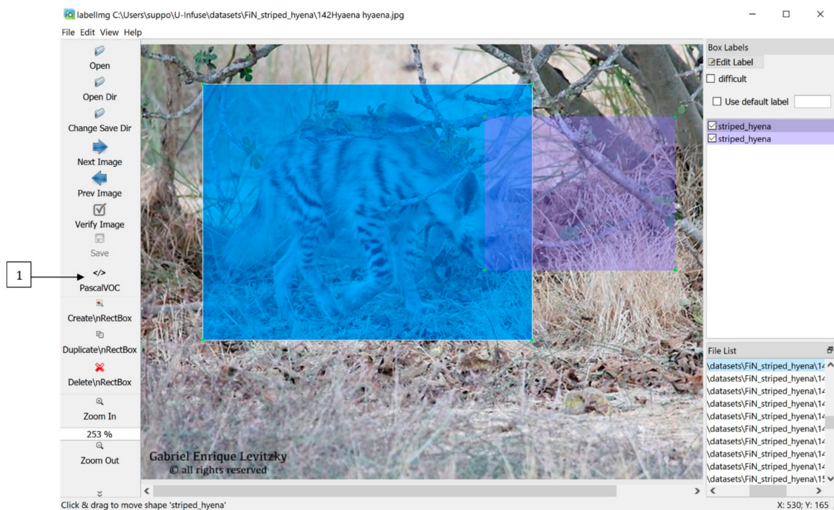
Figure 10. Annotations can be edited in labellmg. Bounding boxes can be added, removed or altered. Labels can also be altered.
