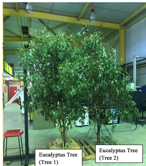
Figure 6. Two trees (Tree 1, Tree 2) positioned in series in between the transceivers.
