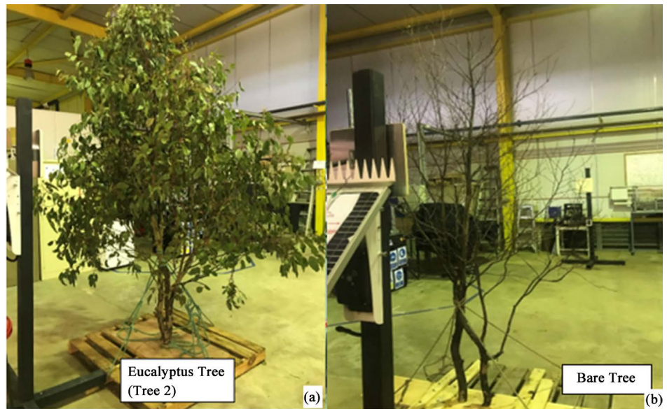
Figure 5. (a) Tree 2 with leaves and (b) Bare tree positioned in between the transceivers.
