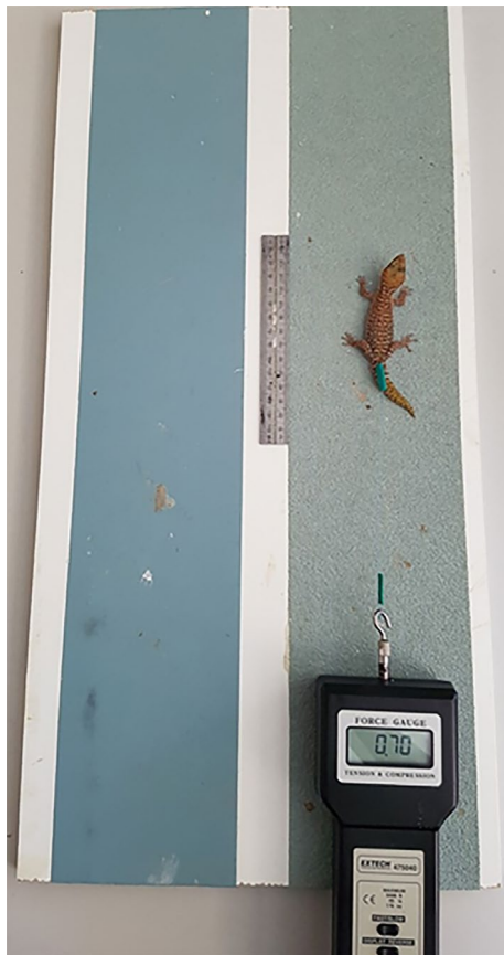
FIGURE 3 View from above of experimental setup used to measure shear force in the geckos Pseudotrichadactylus australis and Oedura coggeri
