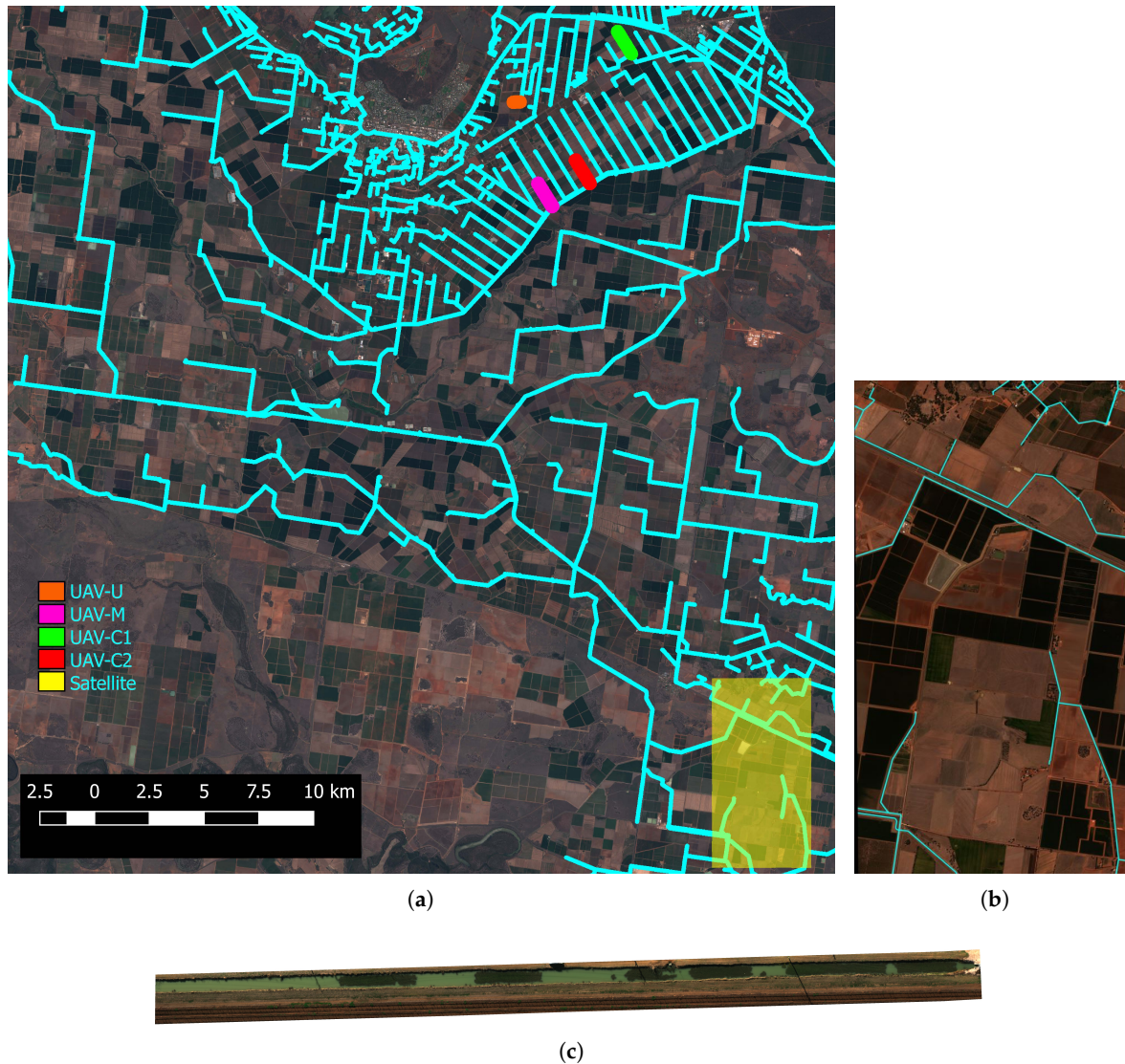
Figure 1. (a) a portion of the Murrumbidgee Irrigation Area with imagery from the Sentinel-2 constellation from 1 Jan 2018. The supply channels are shown in blue. The areas mapped by the UAV and satellite are shown; (b) one of the WorldView-3 satellite images; (c) UAV image of the untreated (U) channel.
