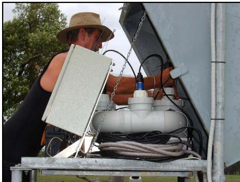
Figure 4.2: The flow-through chamber and sensors of the Greenspan integrated discharge and water quality monitoring system (courtesy CVC).
