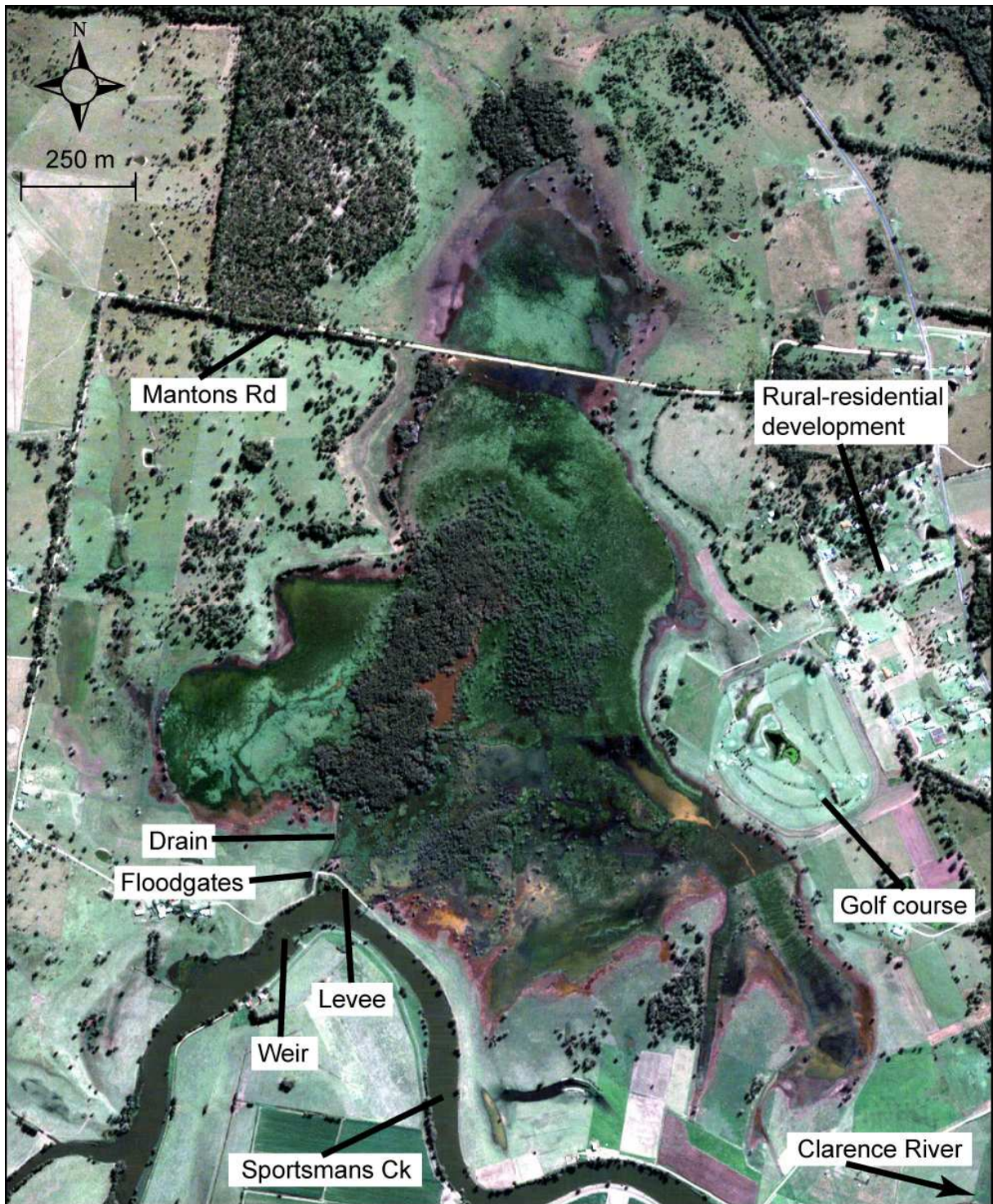
Figure 2.2: Quickbird satellite image (May 2004) of Little Broadwater and local catchment showing the location of flood mitigation structures.
