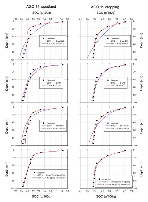
**Figure 4.** Demonstration of how the different mathematical functions (see Table 1) fit the measured data of SOC with depth for a paired site on Grey Vertosols on the Darling Riverine Plain in north Western NSW (Australian Greenhouse Office (AGO) sites 18 and 19).
