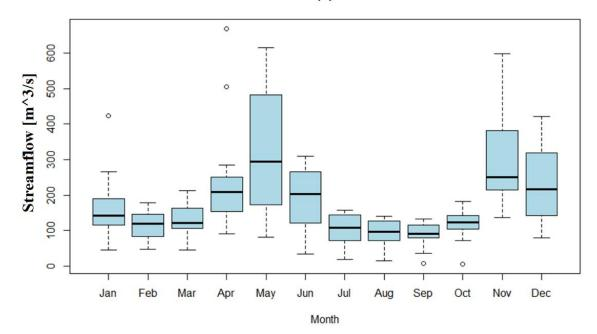
Figure 3. (a) Historical daily discharge measurements and (b) distribution of median monthly Tana River streamflows (period 2000-2016) based on daily readings at Garissa gauging station. Outliers are denoted by "°".
