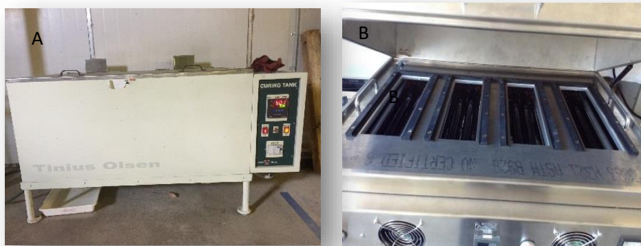
Figure 3.9: Moisture tank (A) and UV-irradiation chamber (B) used for accelerated weathering tests
