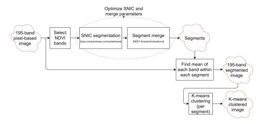
**Figure 3.** Finding optimum parameters for segment generation, and using the segments to create segmented and K-means cluster images.
