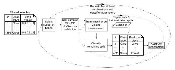
Figure 7. Selecting optimum supervised classifiers and parameters per band combination.
