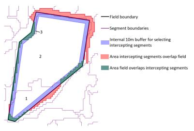
**Figure 4.** Assessment of generated segments against a polygon outlining one of the 75 test fields. In this example, the total area error is the sum of the area of the red and green shapes, and there are three segments intercepting the polygon outlining the field.
