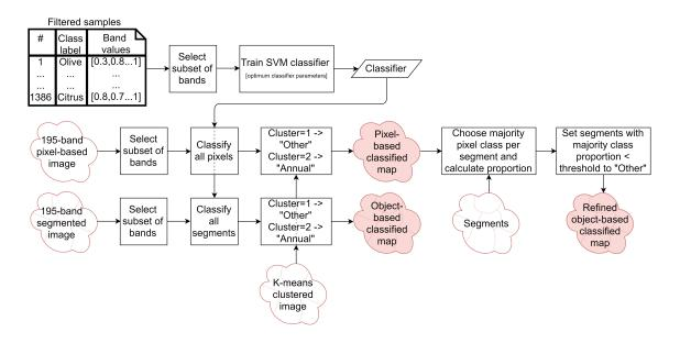
Figure 8. Method of generating pixel-based, object-based and refined object-based maps.
