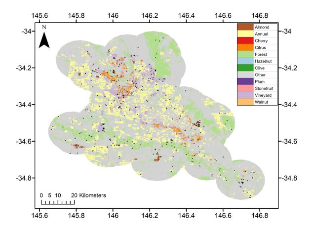
**Figure 16.** Final classified map using S2(10) + S1(2) time series features, and a majority pixel proportion threshold of 60%. The location of the detailed maps in Figure 13 is indicated by the black inset rectangle, and points show the location of the validation segments.
