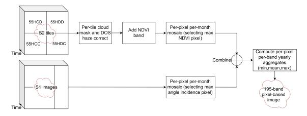
Figure 2. S1 and S2 image preprocessing method.
