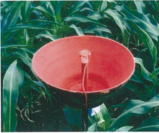
Figure 8.5 Marking zap trap with red dye. Note that dye has spread all over the inner surface of the trap.
