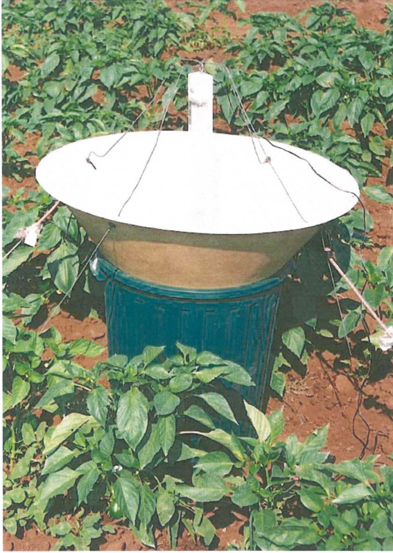
Figure 9.12 Light trap in capsicum. The full setup used in monitoring also had a 30W solar panel to recharge the 12V batteries.
