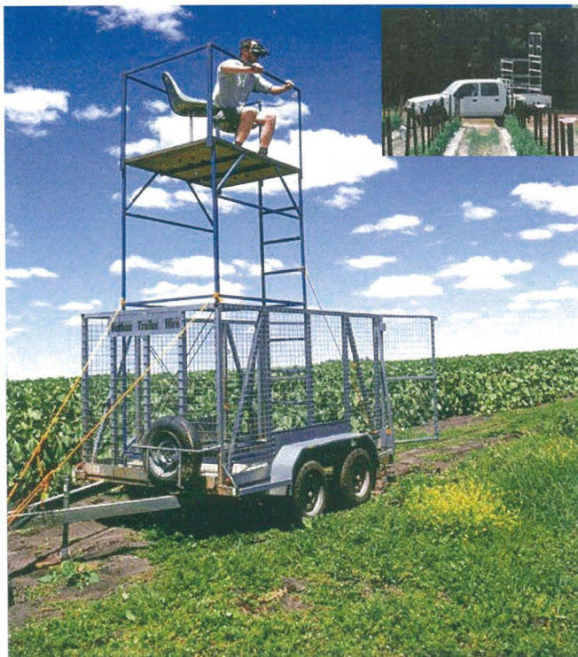
Figure 2.2 The two towers used for night observations for this study. The welded steel frame tower was a fixed height of 4 m (main photograph), whilst the scaffolding tower could be adjusted between 2 and 4.5 m high (insert).
