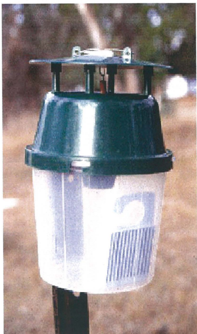
Figure 2.3 Dry or universal funnel trap ("AgriSense trap") showing pest strip in base. Traps used in this thesis had an opaque green base rather than the clear base shown here.
