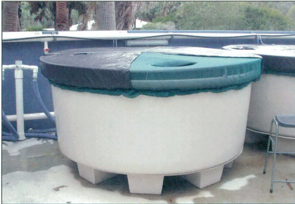
Plate 3.3. The 2 m diameter tank used for each trial.
