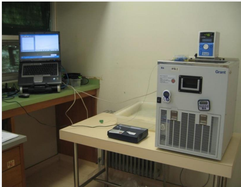
Fig 4. The water bath was connected to a computer which programmed the ramp of temperature at a different rate
