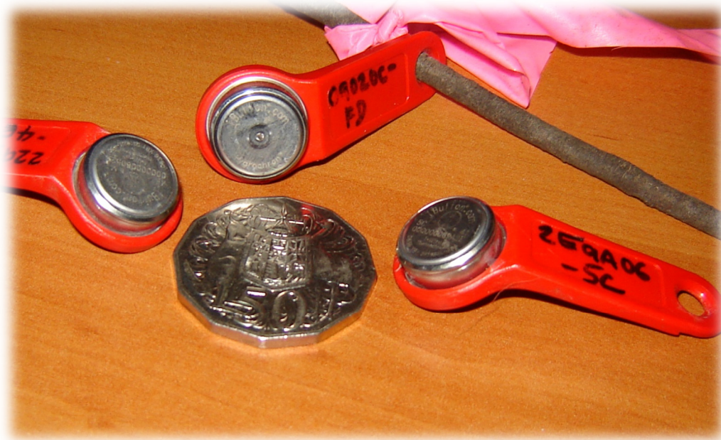
Figure 3: Three iButtons placed in tussocks at each sampling site, the middle one with a hole can measure humidity in addition to temperature
