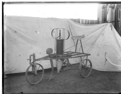
Figure 14-2 "Toxicon" rabbit poison distributor, made by The Clyde Engineering Co. Ltd, Granville, New South Wales, Australia, 1900-1945. Reg. 88/297-578. Source: Powerhouse Museum
