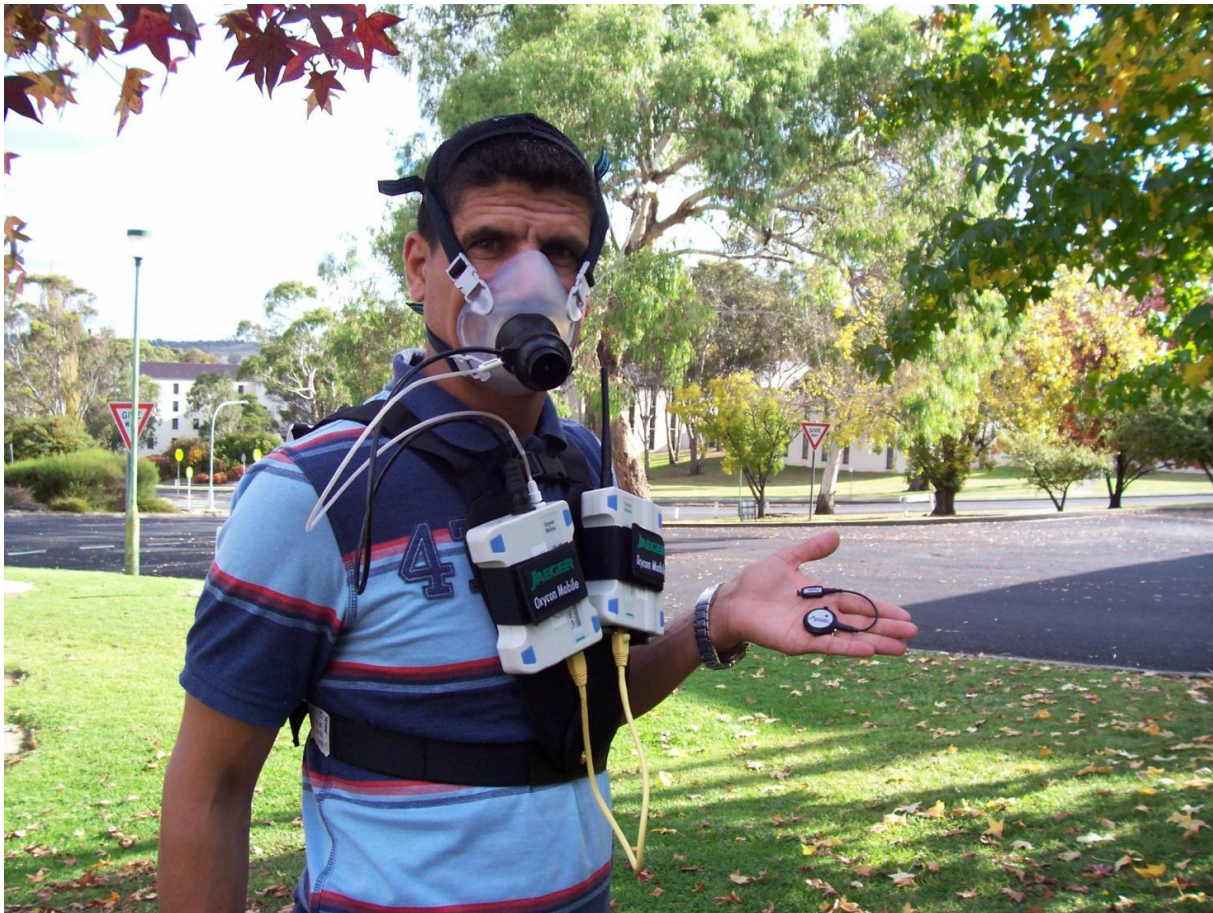
Figure 2-1: The author wearing the Oxycon Mobile system and holding the Actiheart system in his left hand. Note the difference in size and bulkiness of these two pieces of equipment.
