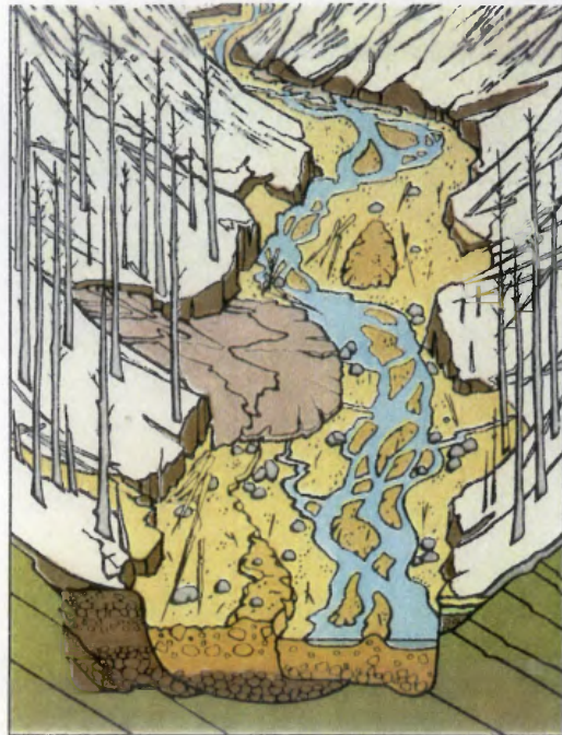
(b) After the 1980 eruption, debris from the volcano ripped up the lag gravel and destroyed the vegetation, causing the hill slopes to destabilise. The stream channel clogged with sediment, straightening the stream course and undercutting and destabilising the banks.
