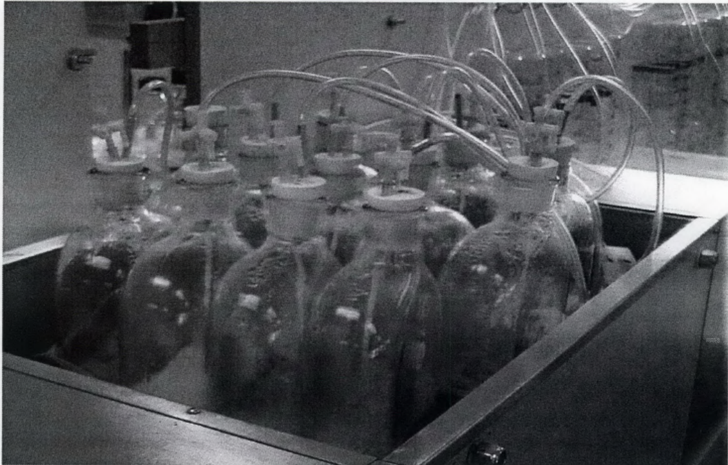
Figure 2 Apparatus used for in vitro incubation of duckweed with rumen fluid. Incubation bottles (volume 1 litre) were held in a shaking water bath and tubes passing through the bungs in each bottle were connected to 500 ml measuring cylinders to enable gas production to be determined by a liquid displacement technique.
