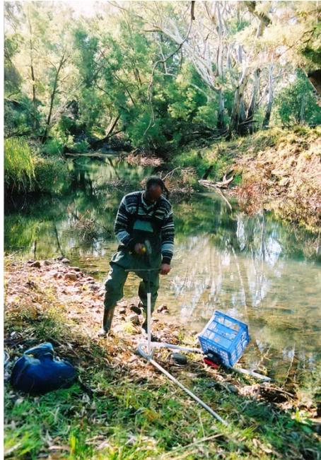
Figure 2.1. Demonstration of the Bou Rouch Pump by Dawit Berhane used to sample Psammaspididae in the hyporheic zone in Maules Creek, NW NSW.
