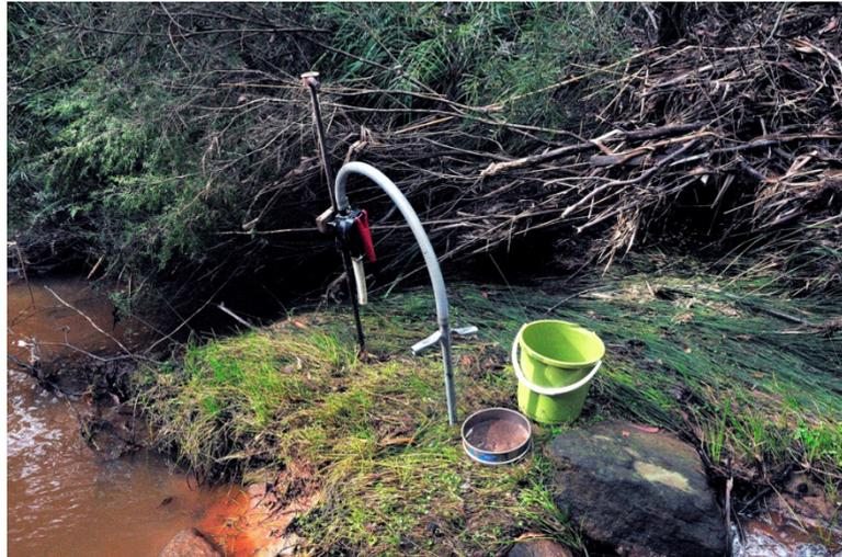
Figure 2.3. Bou Rouch pump set up for sampling the hyporheic zone of streams.
