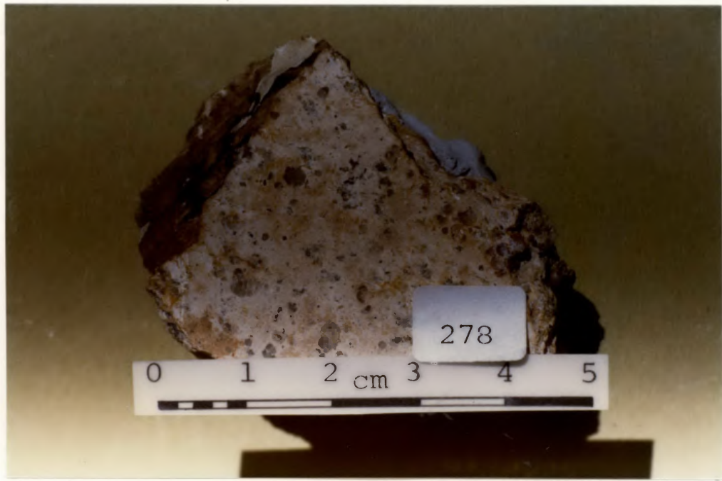
Plate 28. Silica-cemented sorted clasts (1-2 mm subrounded quartz clasts, sand matrix, cryptocrystalline cement, uneven fracture). Uneven fracture through clasts indicates strong cementation (Dumaresq sheet GR 627304).
