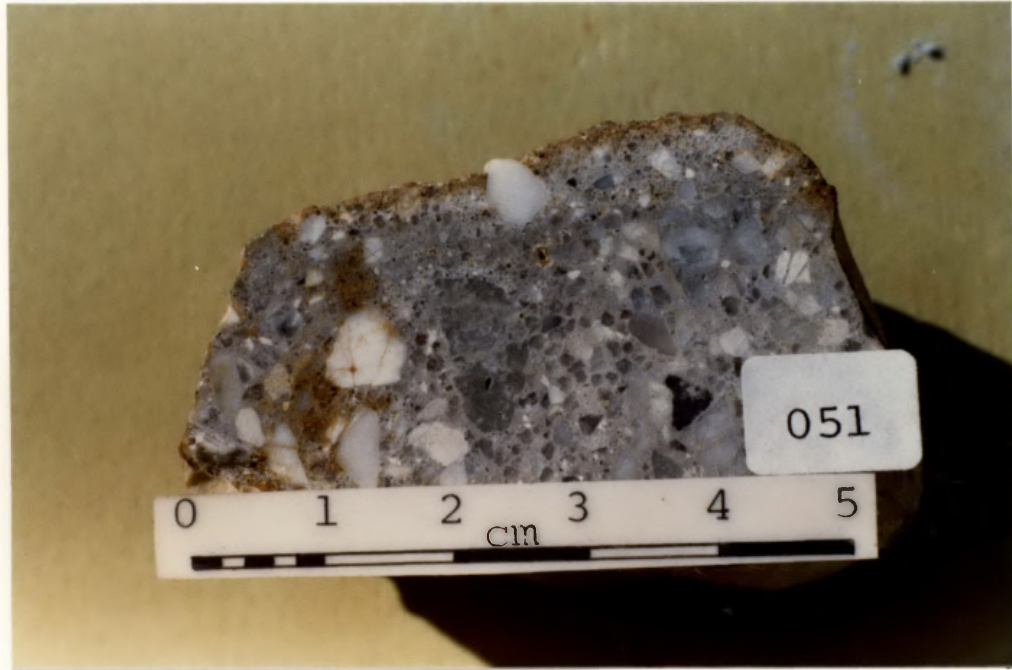
Plate 26. Silica-cemented poorly sorted clasts (0.1-0.7 mm rounded quartz clasts, sand matrix, cryptocrystalline cement). Darker grains are quartz and chert. Sample is from site near Sample 056, within an extensive area of variably cemented, silicified and ferruginised sediments (Armidale sheet GR 656227).
