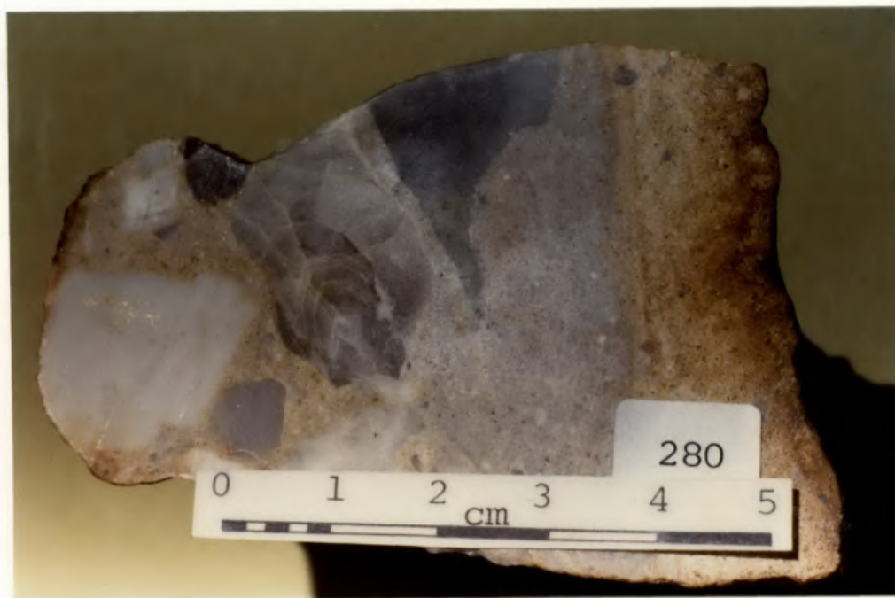
Plate 24. Silica-cemented poorly sorted clasts (0.5-2 cm quartz clasts, quartz sand matrix, cryptocrystalline cement). Rounding of some clasts suggests transport in stream prior to silicification. Zoning in large quartz clast is almost certainly the result of successive stages of crystal growth, and is not related to silicification. (Dumaresq sheet GR 674266).
