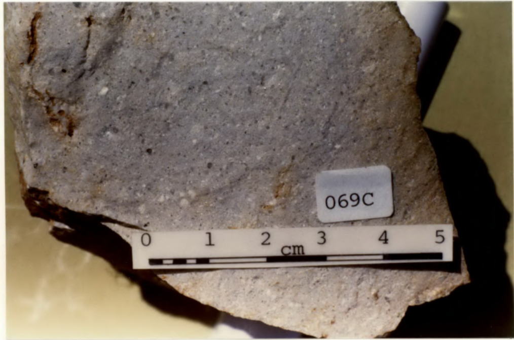
Plate 22. Silica-cemented sorted clasts (0.1-0.3 mm rounded to sub-rounded quartz sand, cryptocrystalline cement, smooth subconchoidal fracture). Dark grains are larger quartz clasts (Armidale sheet GR 598159).
