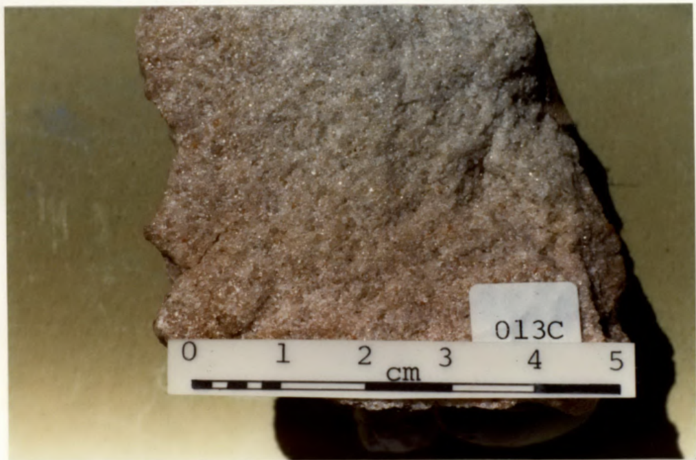
Plate 23. Silica-cemented sorted clasts (0.1-0.3 mm rounded quartz sand, cryptocrystalline cement, 'sugary' fracture surface). Distinctive fracture surface is the result of incomplete silicification (Gostwyck sheet GR 608070).
