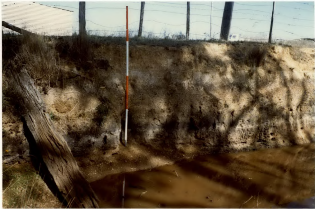
Plate 51. Ferricrete horizon 300 m west of site shown in Plate 50. The ferricrete is 1.2 m below the ground surface, and there is no pallid zone. At this site the ferricrete horizon appears to have formed in soil derived mainly from the Sandon Beds. Bedrock and relationship to basalt is the same as for the site shown in Plate 50.
