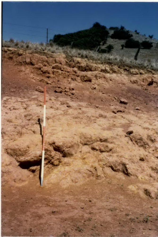
Plate 48. Highly weathered ferricrete underlying relatively unweathered basalt at Arthurs Seat 6 km south of Armidale. The site is 5.5 km east of the eastern boundary of Map 1 (Armidale sheet GR 551199). Traces of spheroidal weathering are visible in the ferricrete near the base of the ranging pole, and suggest that ferricrete may have weathered from basalt much older than the relatively unweathered, 45 m thick, Arthurs Seat basalt.
