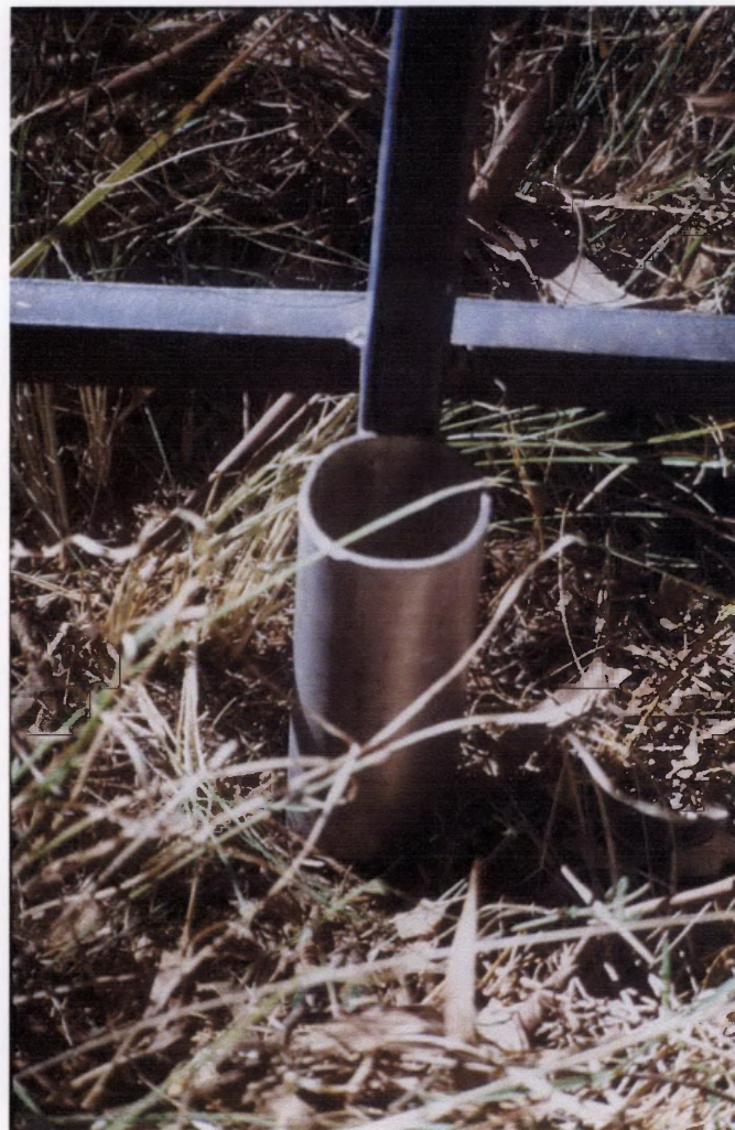
Figure 5.2. Soil corer (5 x 10 cm) used for sampling the soil for seed bank analysis.
