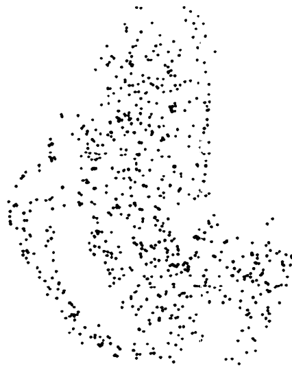
Figure 1.2: A strange attractor calculated by the author using the equation \ddot{x} + 0.02\dot{x} + x(1 + 0.3x + 0.1x^2) = 25 \sin t .
