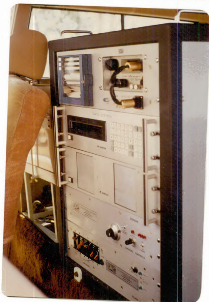
FIGURE 4.5: Vehicle-borne caesium vapour magnetometer and recorders - analog and cassette tape recorders - housed in the car.
