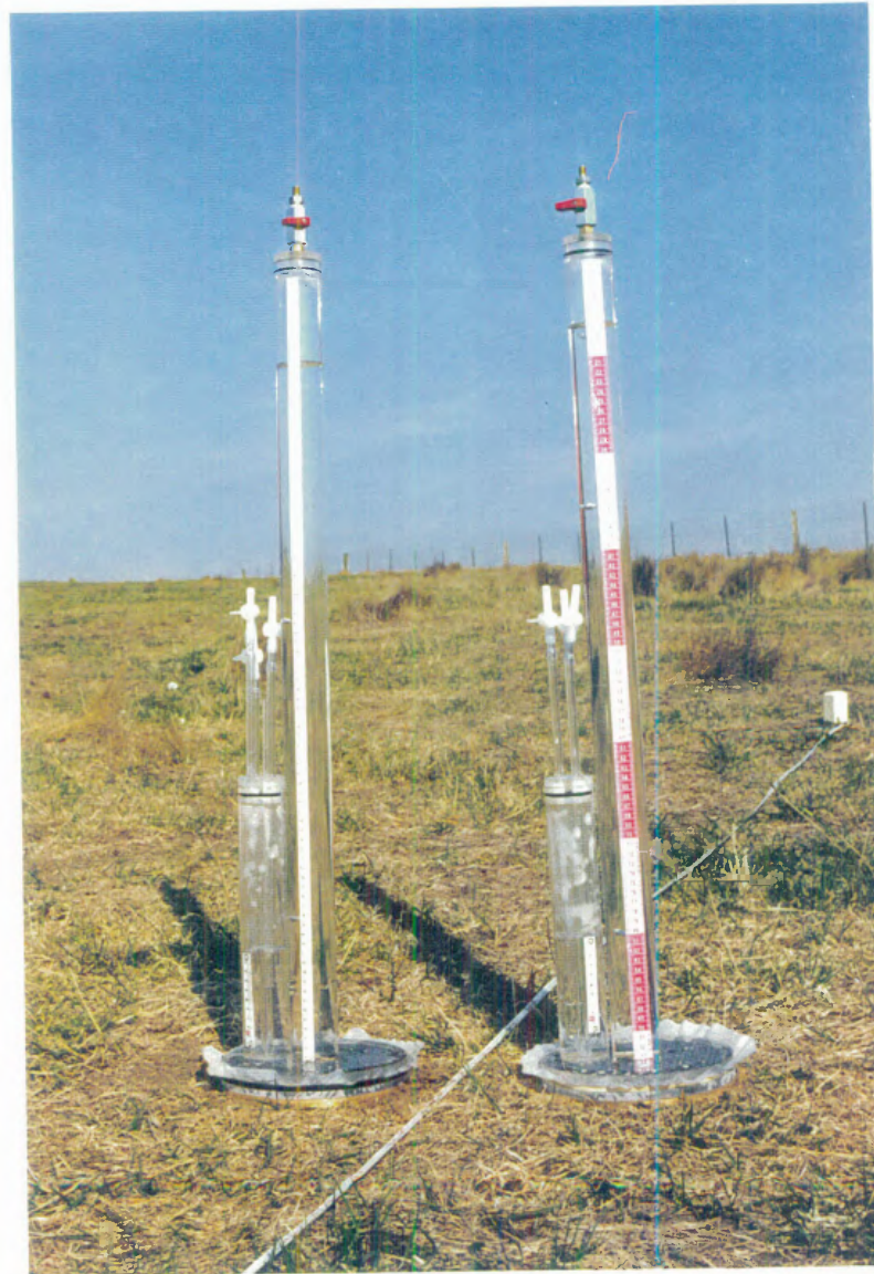
Plate 7.1 The disc permeameters used to determine unsaturated hydraulic conductivity of soils under four tensions.
