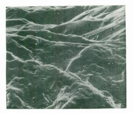
Plate 4 Distinctive glacially generated quartz sand grain surface textures from Krinsley and Margolis (1969)
