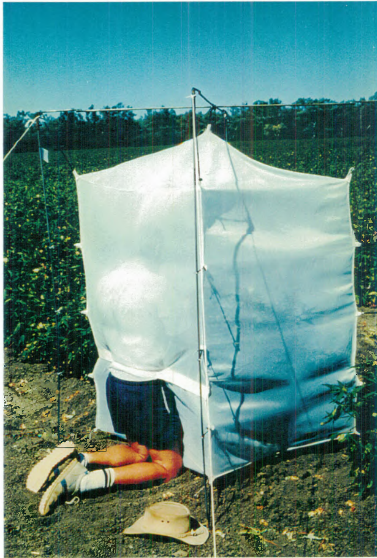
Plate 8. A photograph demonstrating the use of the velcro doors which seal around the researchers waist to prevent the escape of test insects during data collection.
