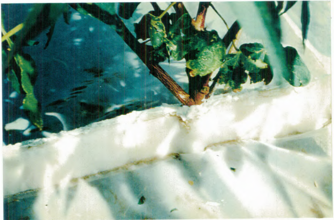
Plate 7. A close up of the floor seal in the field cages to exclude arthropods from the soil. The slit in the suspended floor, through which the plants protruded, were fastened between the plant stems using a 25 mm band of velcro. The top of the velcro join was sealed using a white, non-silicone sealant.
