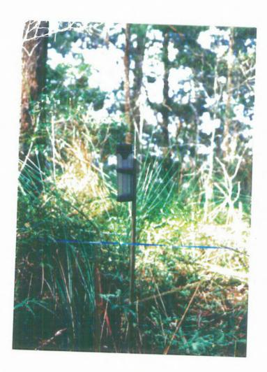
Plate 17. Typical positioning of rain gauge at the edge of the transition zone plot. Plot boundary marking tape can be seen in the foreground.
