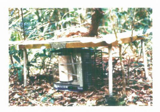
Plate 16. A hygrothermograph in recording position under its protective shelter
