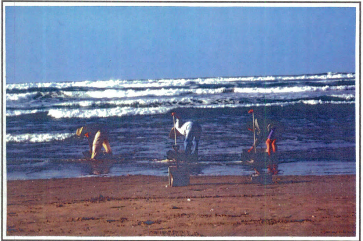
Figure 3.4: Sieving samples through the 1mm mesh using the swash and surf-zone as an aid.
