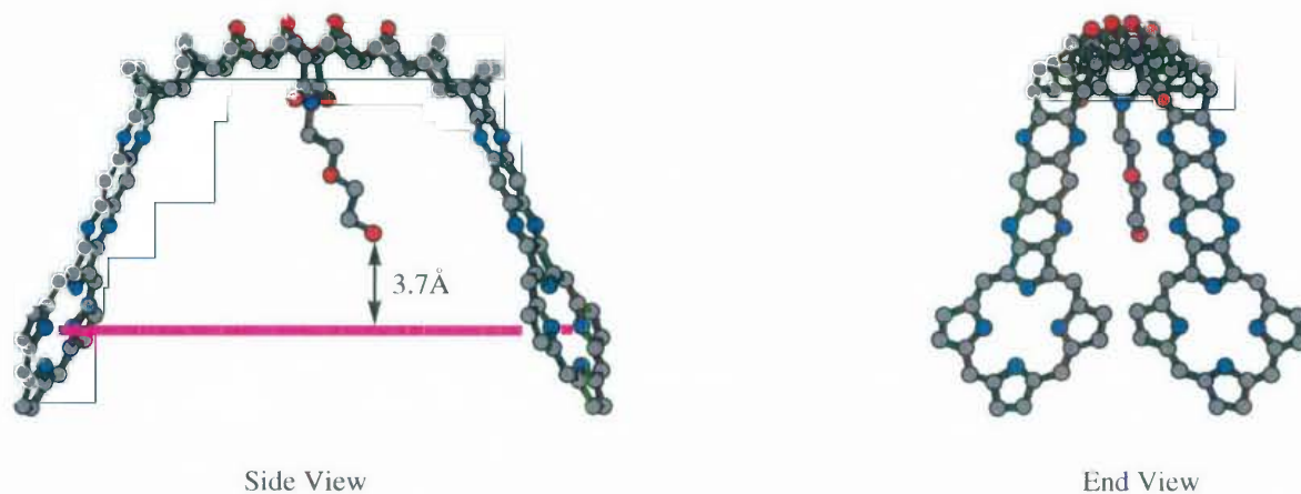
Figure 2.13 Molecular model (AM1) of the skeletal structure of a proposed PSP with a fully extended flexibly tethered hydroxyl group. Static distance (3.7 Å) = the distance between the hydroxyl hydrogen and the interporphyrin plane (pink line).
