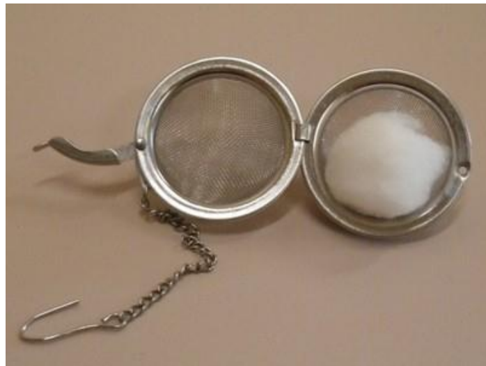
Figure 3.1. Method of presenting olfactory stimuli: a tea infuser (opened) with a cotton ball inside.
