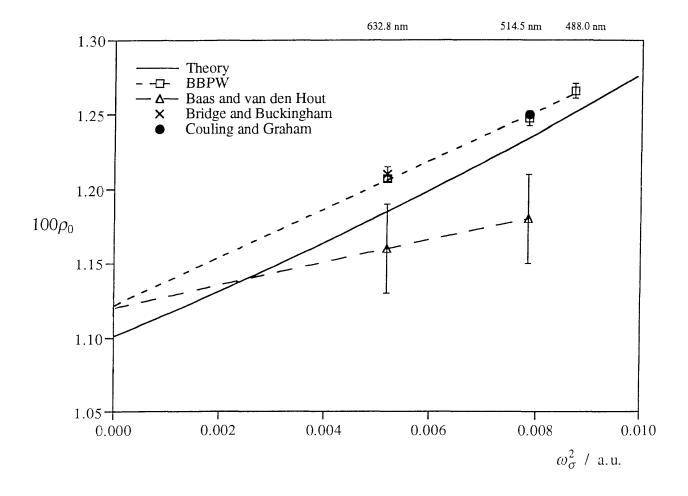
Figure 7.2. Rayleigh depolarization ratios for ethene. The solid line is obtained from pseudo-BD(T) theory with experimental depolarization ratios at dynamic wavelengths from Bogaard, Buckingham, Pierens and White (BBPW) [6], Baas and van den Hout [7], Bridge and Buckingham [8], and Couling and Graham [9].
