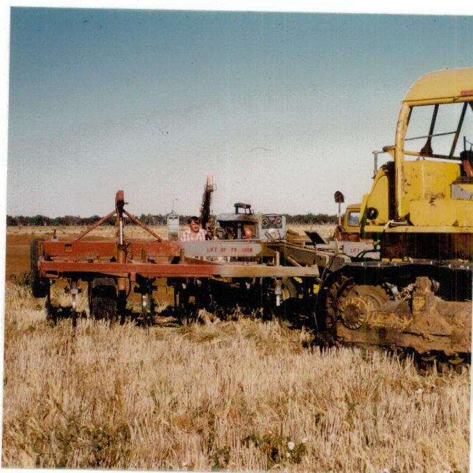
Plate 4.2 Chisel plough tine (left) and chisel plough (above) used to impose experimental treatment.
