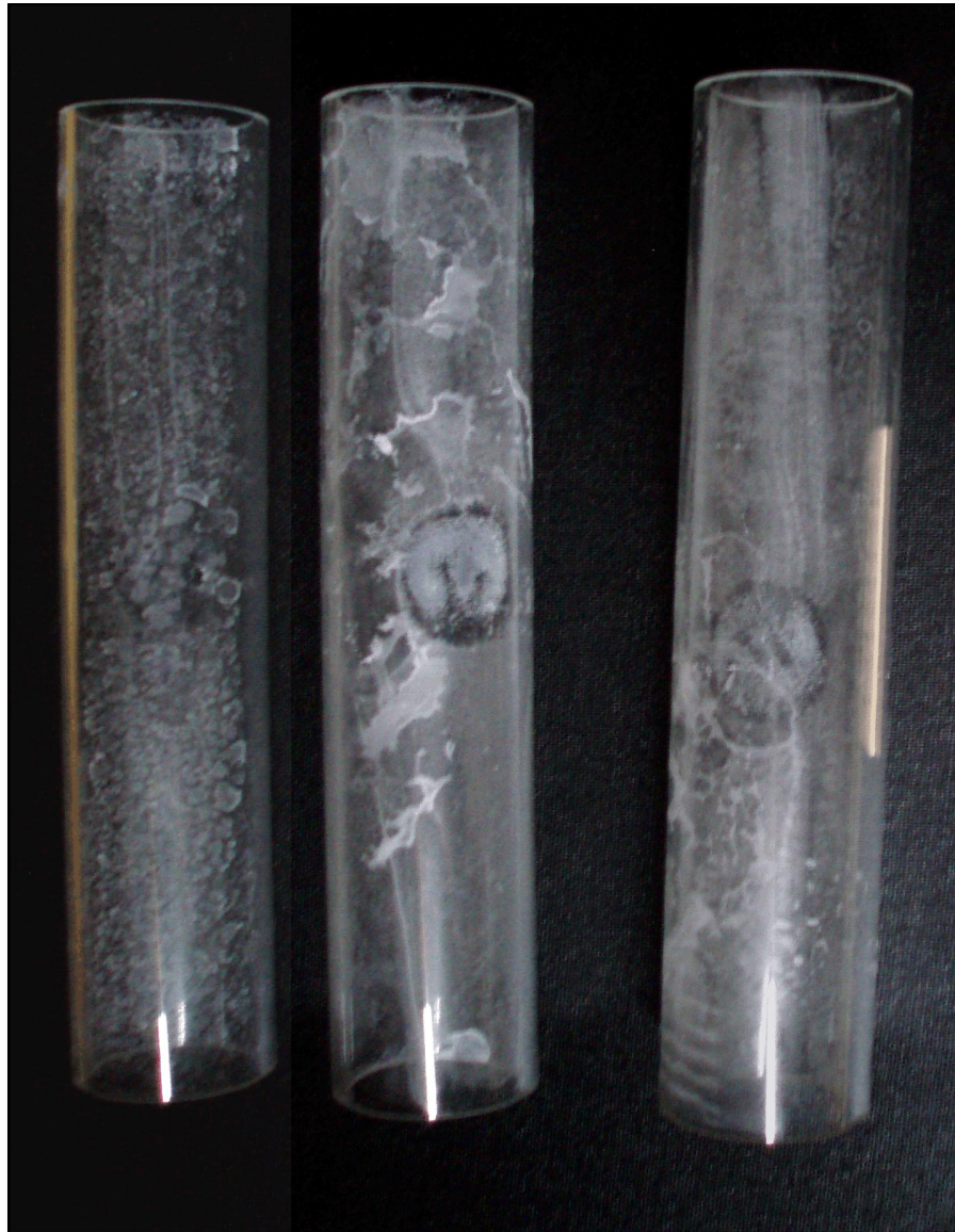
Figure 5.16- The precipitation on the surface of heat transfer tubes in the absence of PAA (blank) for calcium carbonate and calcium sulfate coprecipitation.
